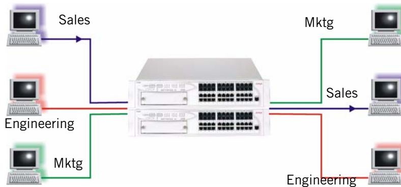
Figure 11.2 VLAN Switching and Bridging
