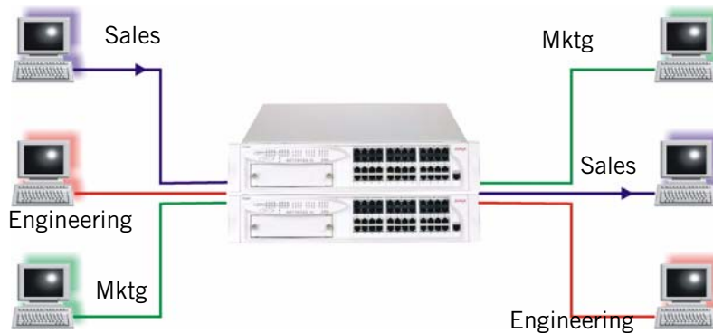
Figure 11.2 VLAN Switching and Bridging
