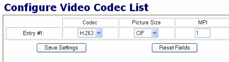
Figure 36: Example of Configure Video Codec List Settings
