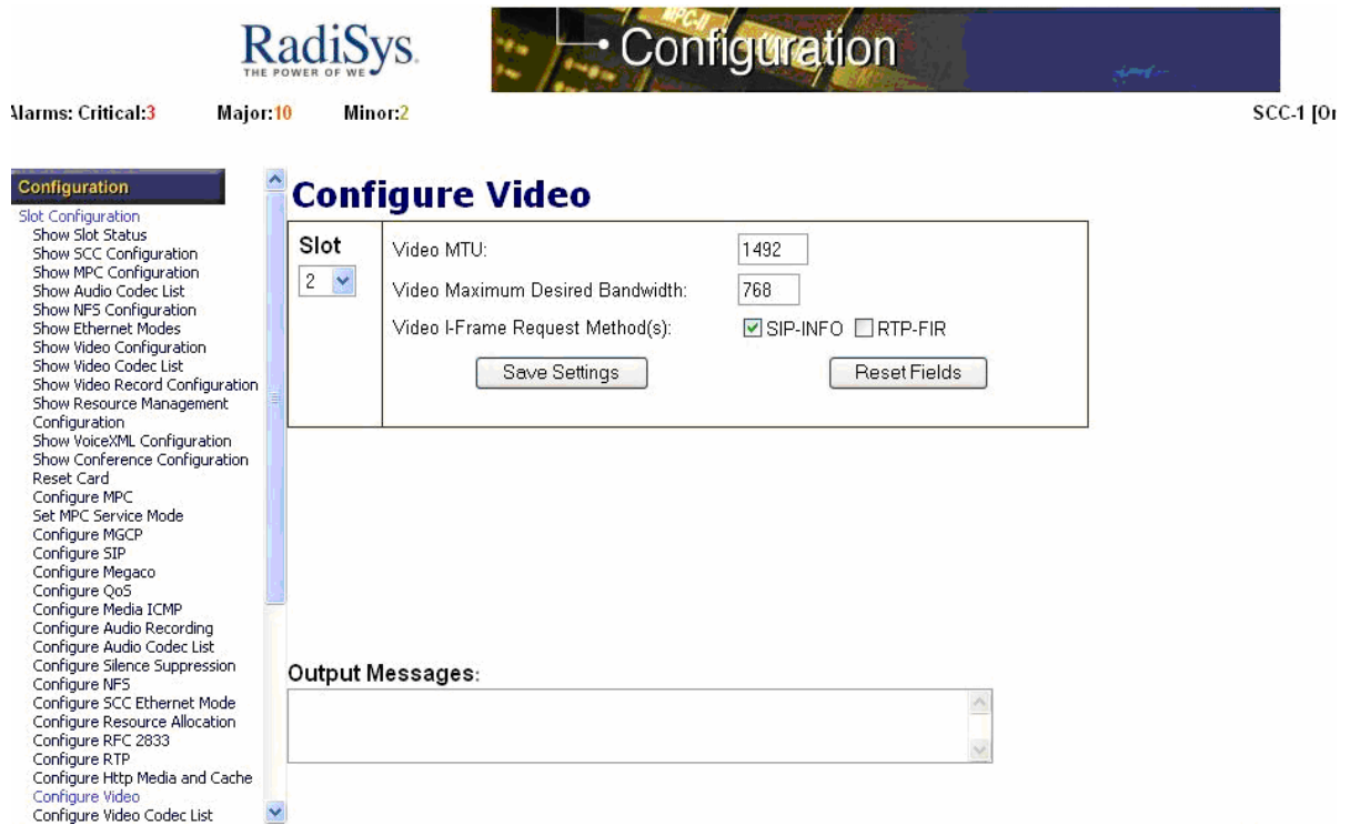
Figure 35: Example of Configure Video Settings
