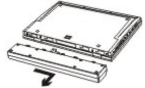
2. Slide the battery pack to the right, and remove.
