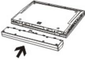
1. Align and insert the battery pack into the corresponding slots on the back of the unit.
