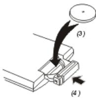
3. Insert a 3V lithium battery into the tray with the polarity ( + ) facing up as marked.
