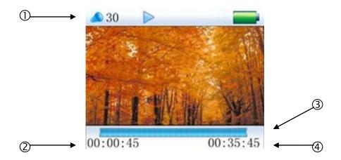
The upper status bar ① contains a numerical volume indicator that you control using the + and – buttons, the play/pause indicator controlled by the >|| button, the position of the video in the current playlist, and battery status. The lower status bar shows progress of the video being played ② in hours, minutes, and seconds, as well as a bar graph ③. The total length of the video in hours, minutes, and seconds appears in the lower right corner ④.
