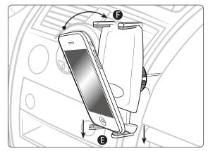
\* If necessary, install the (2) extra long support legs (SP-SM050-LF) to accommodate large sized phones.
