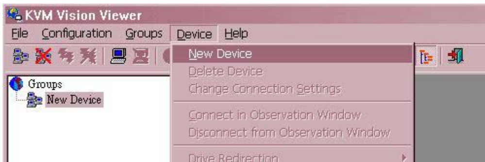
Figure 5-17. Create a new Device
