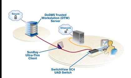
In this diagram, the SwitchView SC4 UAD switch supports the DoDIIS Trusted Workstation and the secondary unsecure workstation with a DVI-I interface, USB keyboard and mouse, and audio peripherals.
