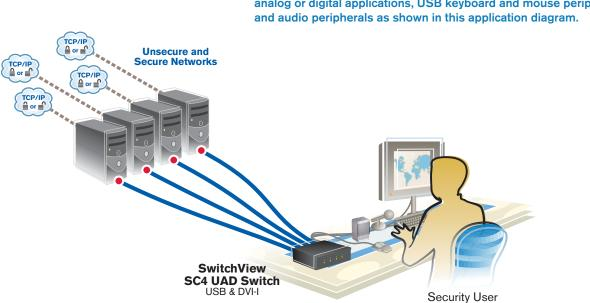
The SwitchView SC4 UAD switch supports DVI-I video interfaces for analog or digital applications, USB keyboard and mouse peripherals,
