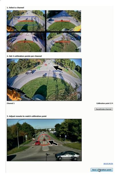
The image shows a snapshot of an ongoing calibration. The arrows point out calibration point 3 in the upper left channel view and the corresponding point in the PTZ camera view.
