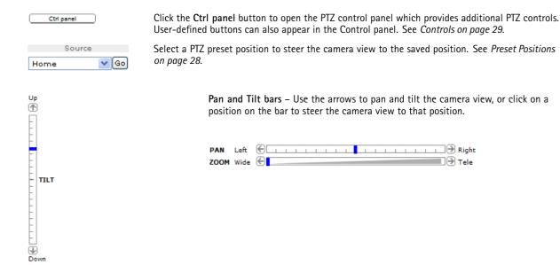
The PTZ controls can be disabled under PTZ > Advanced > Controls, see Controls on page 29.
