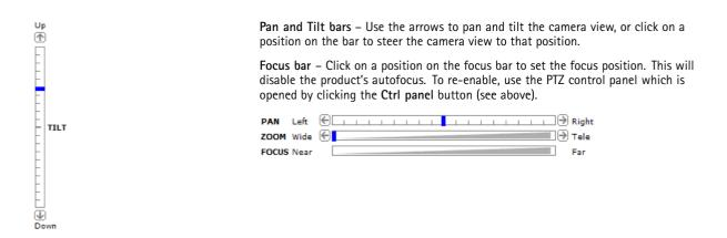
The PTZ controls can be disabled under PTZ > Advanced > Controls, see Controls on page 29.
