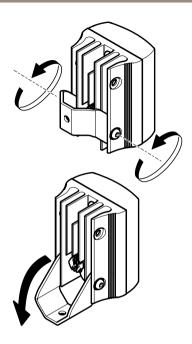
If required, loosen the screws and change to a diverging lens with the desired angle of illumination. The angle of illumination should be adjusted according to the camera field of view to light the whole scene adequately. See *Technical Specifications*.
