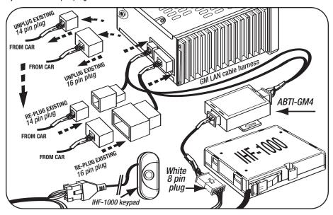
4) Insert the 16 pin plug on the ABTI-GM4 cable into the rear of the radio.
