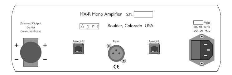
When you have a choice, a properly implemented balanced connection will offer higher sound quality than a single-ended connection.
