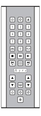
The very bottom button activates the remote handset's backlight, and is placed off by itself so that it can easily be found by feel in a darkened room. The unit is backlit with a special fiber optic array that distributes the light from a single blue LED to the entire keypad. Each button is fully illuminated so that the button's icon can be easily read. The Multi-Component Backlit Remote Control makes operation of your audio system easier than ever.
