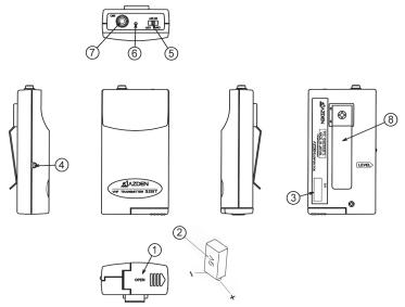
(1) Open the battery compartment lid by sliding it in the direction indicated and raising it.
