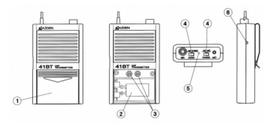
**41BT** body-pack transmitter with 63 on-board user selectable UHF frequencies. Ideal for use with lavaliere and headset microphones. The MP-1 instrument cable will also allow you to use the 41BT with electric guitars and basses. Please note: For use with instruments the gain structure of the 41BT must me modified at the factory.
