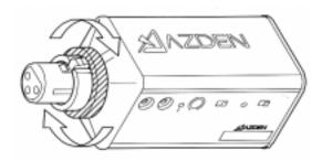
To plug the 41XT onto a microphone (low impeadance with XRL connector) first make certain the the locking-ring is turned fully up (rotate counter-clockwise). Then plug the 41XT fully into the microphones XLR connector and tighen by rotating the ring fully down (clockwise).
