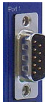
Figure 8. DB-9 Female Serial Port Connector
