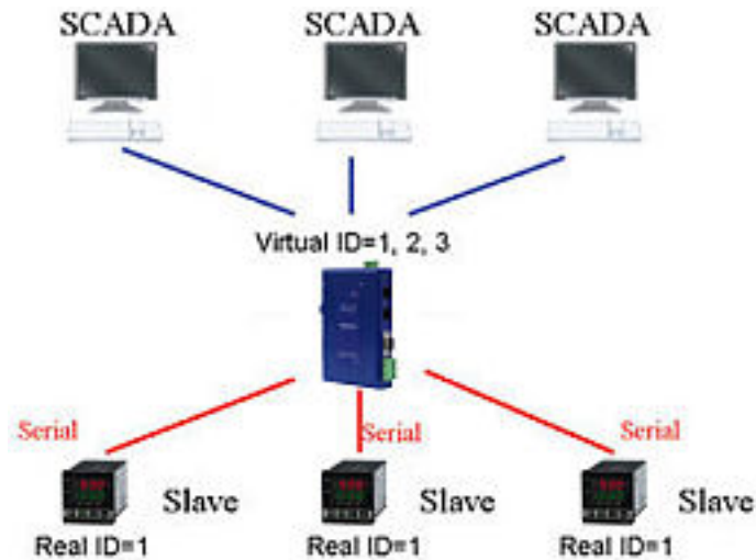
Figure 25. Scada to Slaves, IDs Fixed
