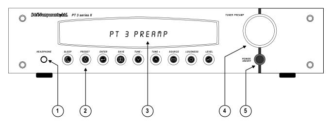
**1. Headphone Jack** - Stereo headphones having a standard <sup>1</sup>/<sub>4</sub> inch binaural plug can be connected to the headphone output. The Preamplifier Tuner must be on and in HEADPHONE Mode for proper headphone operation.
