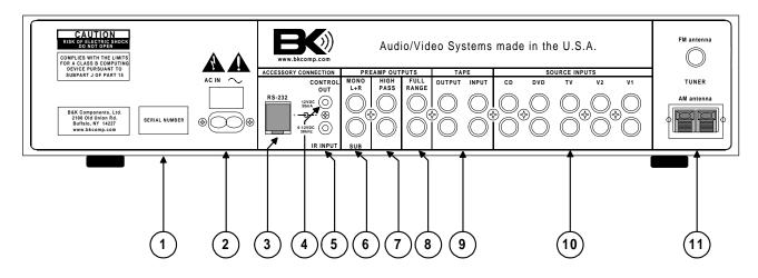
The Preamplifier Tuner's back panel is organized into groups of inputs and outputs as shown below. See back of this manual for an enlarged view.
