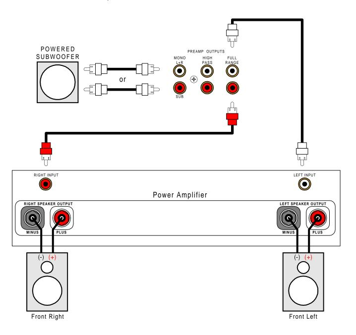
**SUB output -** Connect an RCA cable from the Preamplifier Tuner's SUB output. If your subwoofer does not contain its own amplifier you will need to purchase an external B&K or other power amplifier. Connect the Preamplifier Tuner's SUB output to the audio input of the external amplifier. Connect the external amplifier's speaker output to your subwoofer. If you prefer to use your subwoofer's internal crossover, connect to the Preamplifier Tuner's Mono output.
