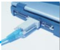
CAT5 Network Cable
