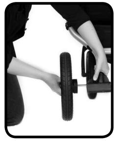
**1** To install, gently slide the rear wheel's axle into the hole in the frame until the wheel clicks into place.
