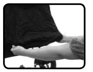
• Weather Cover: If desired, pull weather cover down and over the seat back mesh. Secure firmly over both sides of seat. When not in use, roll weather cover up and fasten with elastic loop and barrel provided under top of the seat fabric.
