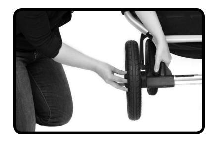
**2** To remove, simply press the wheel button while gently sliding the wheel away from the frame.
