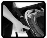
• To release parking brake: Pinch gray tabs and pull towards you. Push brake lever down until it is parallel with the frame.
