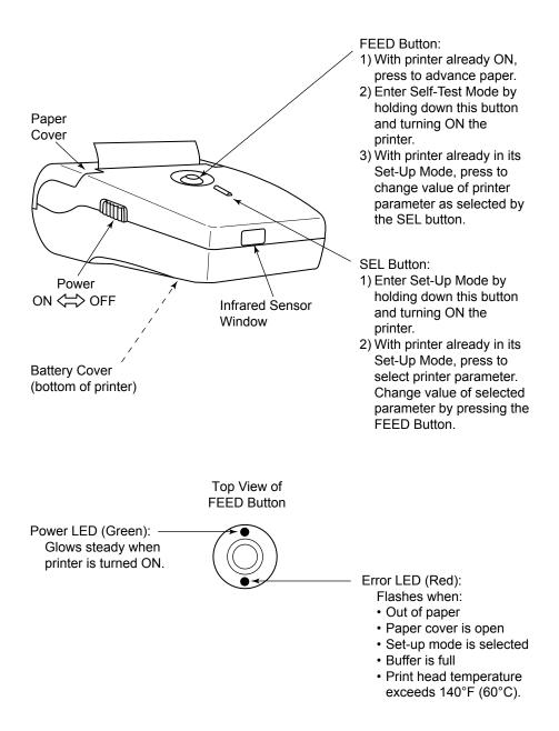
Figure 1. Component Locations and Functions
