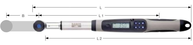
**Calculation of the compensating** torque when using an extension A torque wrench is typically adjusted and calibrated by applying a known force at the center of the handle at a distance L1 from the center of the driving square.
