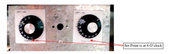
This will provide a cabinet air temperature of between 75-80°C.
