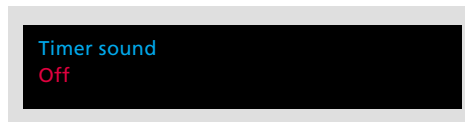
The Timer menu – the Off or On options decide whether sound is to be distributed to the TV speakers from a Timer play that you have made on your audio system, which must be connected to your TV.
