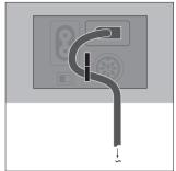
Cable clamp: For safety reasons, the mains cord from the wall outlet must be secured to the loudspeaker. To do so, tug the cord behind the clamp.
