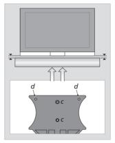
Adjustments: First, make sure that the television is adjusted to a level position on its stand or wall bracket! Then use the two screws (d) to adjust the loudspeaker so that it is parallel to the lower edge of the television. Align the loudspeaker front with the television and tighten the two screws (c).
