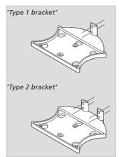
BeoLab 7 brackets: The loudspeaker must be fastened to one of the brackets shown here, and on a suitable Bang & Olufsen stand or wall bracket.
