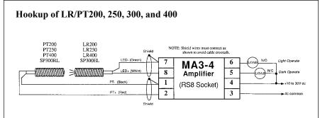
NOTE: Shield wires must be connected as shown to avoid cable crosstalk.
