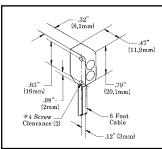
SP300D: the SP300D is the diffuse mode version of the SP300L with the same rugged aluminum housing and totally encapsulated construction. The glass lenses are hermetically sealed, which eliminates any possibility of condensation inside the lenses and allows operation in adverse environments like steam washdown and high vibration. The SP300D may be mounted by its throughholes or with the SMB300 bracket, as shown below.
