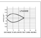
sensing objects with irregular surfaces (e.g.- webs with "flutter"). The optics are such that even small threads or wires .005" (0,1mm) or greater in diameter may be detected when they pass within .25" (6mm) of the sensor's plastic lens. Due to its wide response pattern, the LP400WB should not be used for precise positioning control, nor should it be mounted with its lens recessed into a hole.
