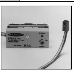
**ADJUSTMENT:** GAIN adjustment (single-turn potentiometer; adjust with small flat-blade screwdriver).
