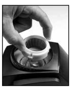
Pull the silicone seal off the top of the ring Burr. Remove the ring burr by lifting it straight up out of the grinder by the lifting tabs. If the burr does not lift out, ensure that the grind adjustment tab is turned fully counterclockwise.
