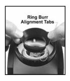
After replacing the burr, replace the silicone seal by lining up the two slots in the silicone seal with the small tabs on the top of the ring burr and slide the seal onto the ring burr.
