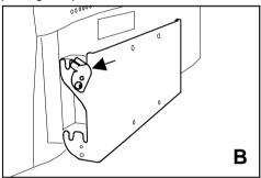
Step 3: Place the panel on the mounting plate
