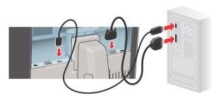
3 If you want to make use of your display's USB downstream connectors, connect a PC USB downstream connector to the display's USB upstream connector by means of the supplied USB 2.0 cable
