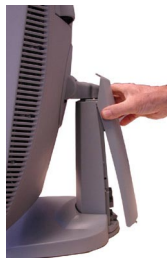
Push the upper side of the cover onto the foot
