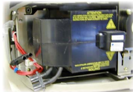
Image 3-9 disconnected lamp connector
