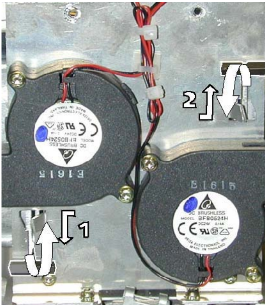
Image 3-13 locking lamp 1 & lamp 2
