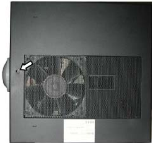
Image 4-1 Location of side door screw
