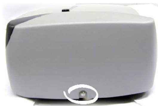
Image 3-5 rear cover lock screw
