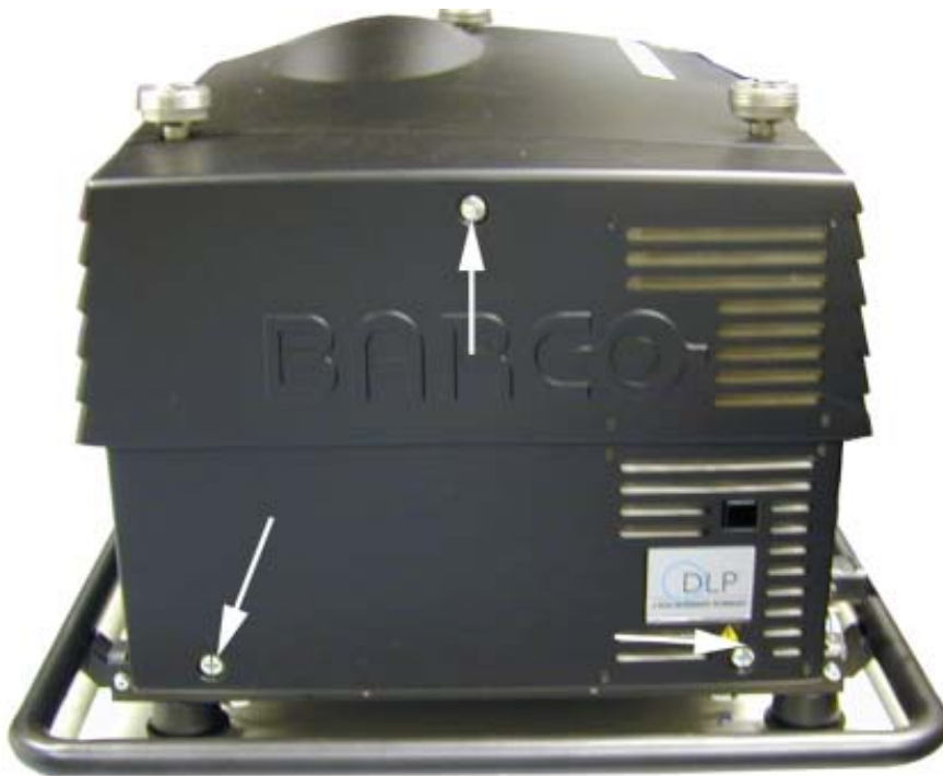
Image B-6 Back cover removal
