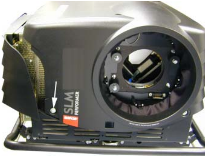
Image B-3 Front screw top cover removal
