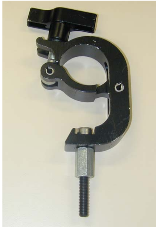
Image 3-31 Closing the rigging clamp
