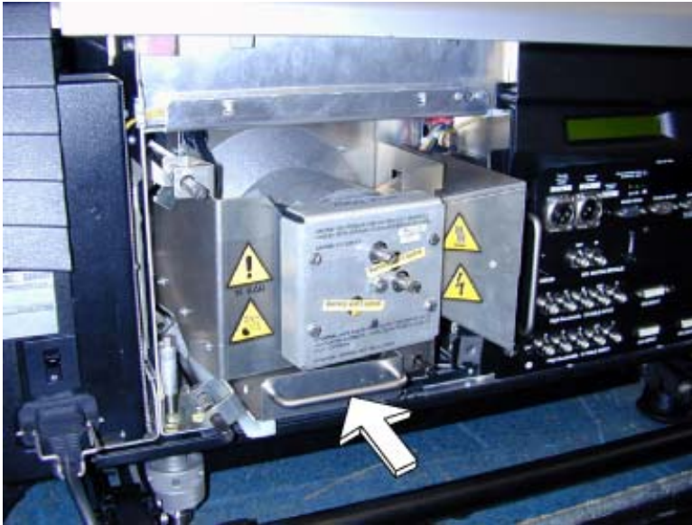
Image 3-10 Inserting the lamp
