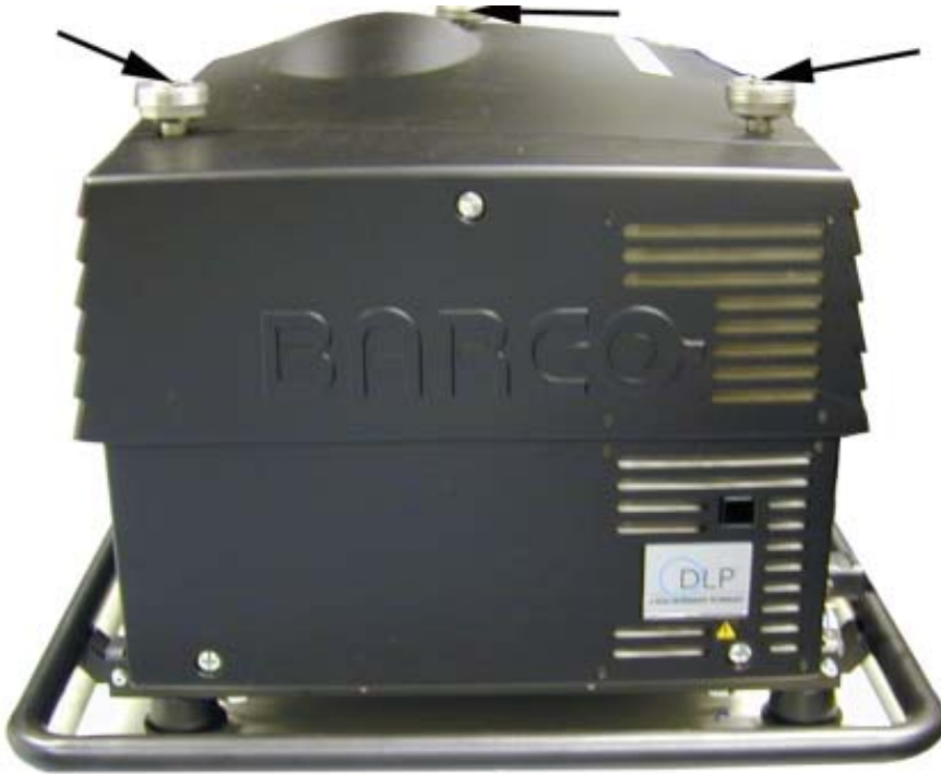
Image B-1 Removing stacking sockets
