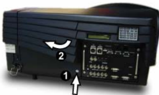
Image 3-15 Lamp adjustment access
