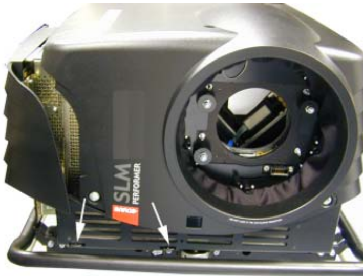
Image B-9 Dust filter bottom side
