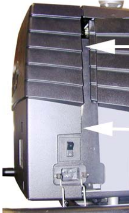
Image 3-12 Mounting the side cover
