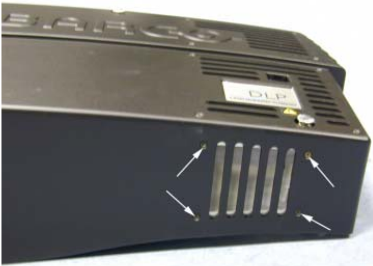
Image B-8 Dust filter removal
