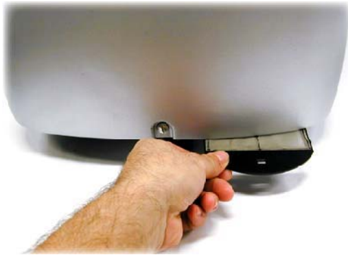
Image 15-3 Lamp filter removal
