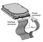
**Note.** You can mount the drive in any orientation. Usually it is mounted with the circuit board down.
