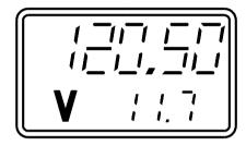
The supply voltage is continuously measured. Indication occurs only in mode 3. The mode is selected by briefly pressing the MDE key once or several times (corresponding to the previous state) the active frequency on which the VHF station is ready for operation is shown in the top line and the measured voltage is displayed in the bottom line.
