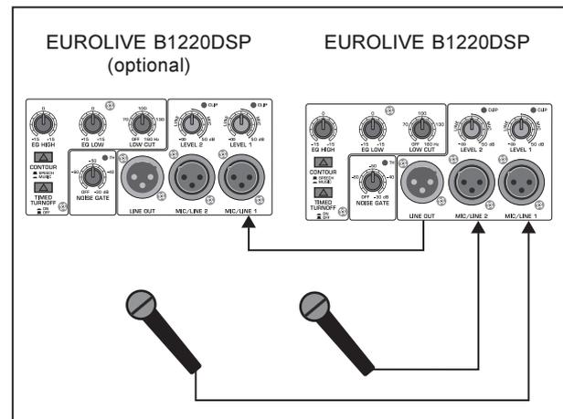
Fig. 4.1: Connecting microphones
