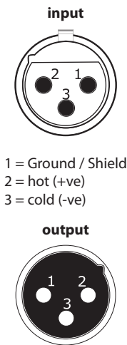
Fig. 10.1: Un-/balanced jack plugs and balanced XLR connectors
