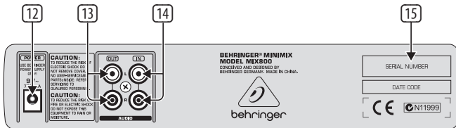
Fig. 2.2: Rear panel connectors of the MIX800
