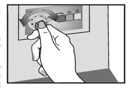
temperature of approx. 32°C, the thermostat should be adjusted to the mild position.
