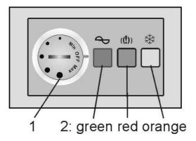
The indicator light set is placed on the front side of the freezer for easy visibility.
