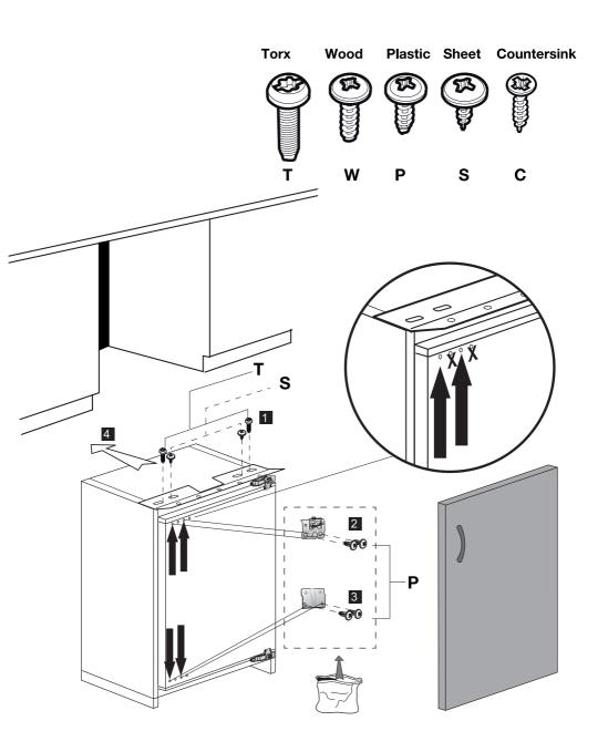
**Note:** Installation step for 2, screws for connecting top plastic rpart should not be screwed very hard, because of moving the plastic part easily left or right side.
