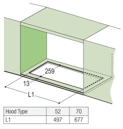
Make a rectangular opening on the base of the hanging unit, leaving a minimum of 13 mm from the outer edges.
