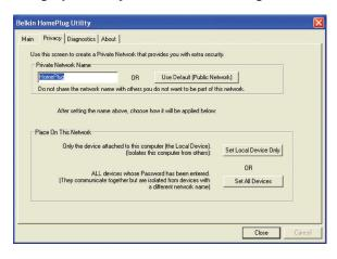
The "Privacy" tab allows you to change the network password to the unit that is currently connected to this computer. This network password encrypts all data that is sent from this unit using 56-bit data encryption standard (DES). The DES encryption is very secure and difficult to crack.
