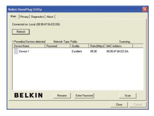
In the following window, enter the DEK located on the bottom of each device into the "Password" field. Note that this password is different from the network password.
