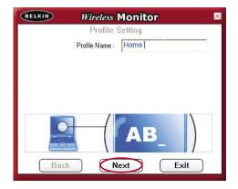
Step 2. The next screen you will see allows you to type in the name of the network you will be connecting to, the type of network it is, and optionally, set the data rate for that network. After making the selections, click "Next" to continue.
