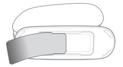
2. After a brief installation, the setup software will ask you for the network name and password from the network information card that is stored in the foot of your new Belkin Router. Store the card under the base of your Router for future reference.
