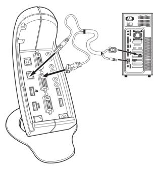
2. Take the DVI cable and connect the male end of the cable to the DVI port on the back of the computer. Connect the other male end of the DVI cable to the back of the KVM Switch for CPU1.
