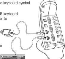
5. Connect any USB devices you wish to share to the USB hub labeled "Device 1, Device 2" on the KVM Switch.
