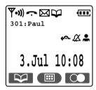
Ψ Within range of a Cell Station **`**\**\** Out of range, No registration •))) Intercom Indicator **Off-hook Status** Message Waiting  $\square$ Phonebook Mode  $\sim$ Battery Strength Ū, Hot Line ON X **Ringer Volume OFF** N Vibration Μ Meeting Mode Call Forwarding ŝ Do Not Disturb •K—
