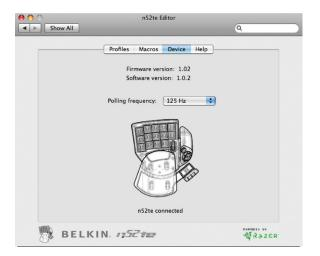
**Firmware Version –** This displays the firmware version of the n52te currently connected to your Mac computer.
